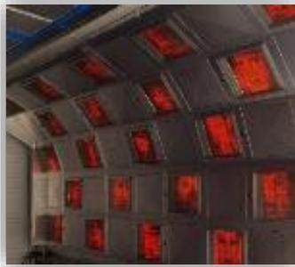
The dimensions of the tunnel oven must be adjusted to suit the product. Thermoreactors® walls of the enclosure structure are made of welded-frames and galvanized steel panels, they can be vertical or adapted.
