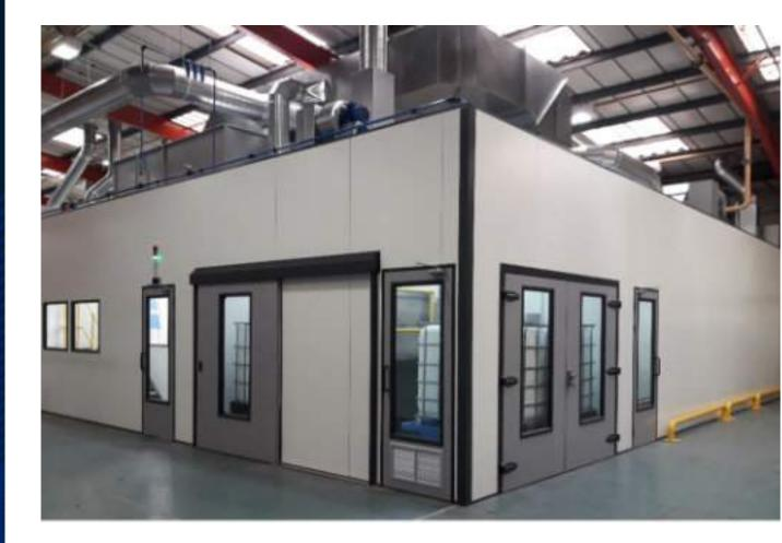
Our client, specialising in industrial and automotive coatings appointed us to provide a full paint facility, comprising of Spray Booth Ovens, Preparation Booths, Ionising Enclosure, box and tunnel. Through our consultative approach Unitech identified that a complex but efficient conveyor system would best meet the needs of the client.
